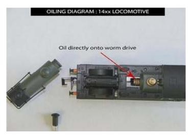
The motor and worm should free off and the locomotive should start running.
