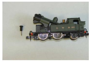
With power applied to the layout, place the chassis on the tack, and gently, with the aid of a small plastic sprue or wooden tooth pick, push the worm to 1 side or the other depending on how free it feels.
