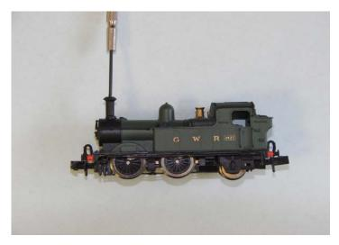
The cure is relatively simple. Firstly unscrew the screw that is found in the chimney. This holds the smokebox and boiler barrel in place between the water tanks. The pull up gently on the smokebox and the boiler barrel will come away exposing the worm within the split frame.
